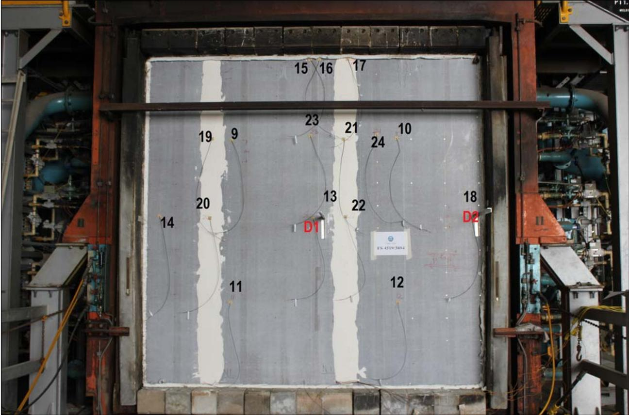
Unexposed face of test specimen detailing external face thermocouple locations
